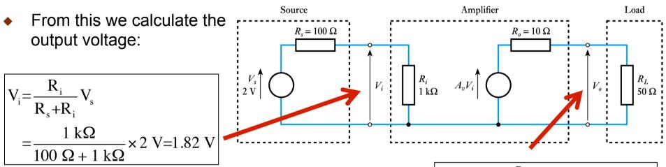
Although the amplifier has a gain of 10 when it is NOT connected to anything, when used in the system, the actual gain is:
